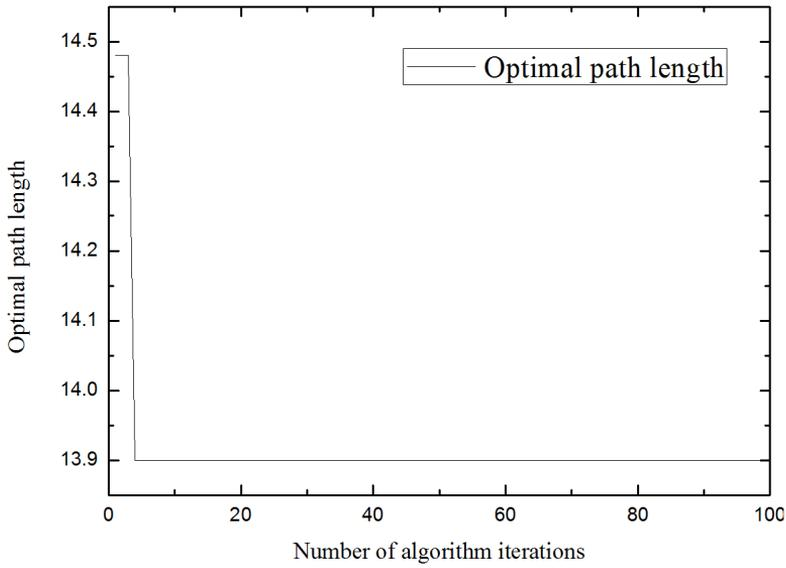
Fig. 5. Optimal path evolution of ant colony algorithm
